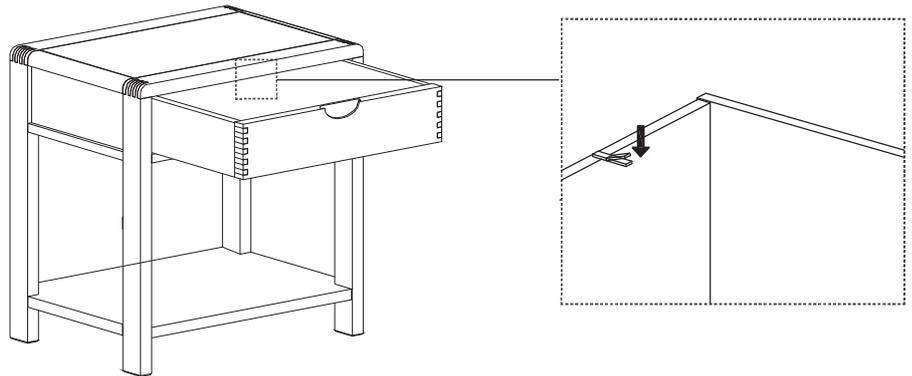
1. Place your product in the final position. Loosen the screws on the metal brackets just enough so that the slotted bracket can be extended to meet the wall.
