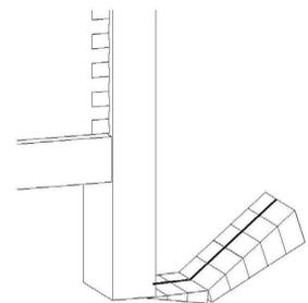
If the chest is not level on your floor, use the wedges provided. Snap them off, so they do not protrude out from the cabinets legs. You can also snap them lengthways. See diagram right.
