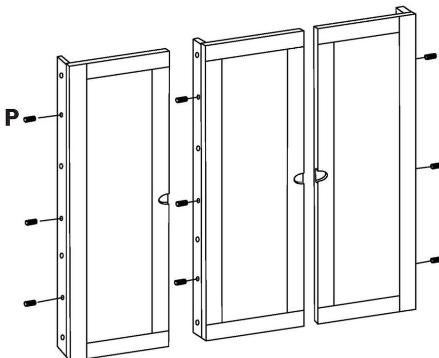
5. Fix the door frame(I) onto the side panels(B&C) and centre panel(D) using the 25mm screws(M) 12pcs as shown below.
