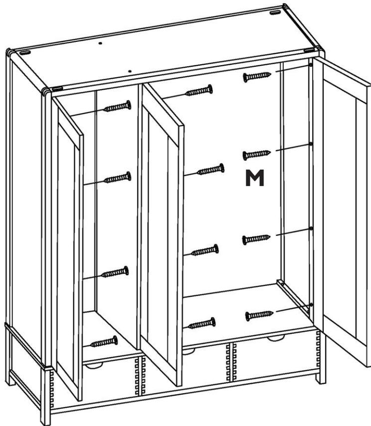
6. Push fit the eight shelf pins(Q) and locate the self (J) using 16mm screws(L) 8pcs as shown, Put the hanging rails(F&G) into their rail supports.
