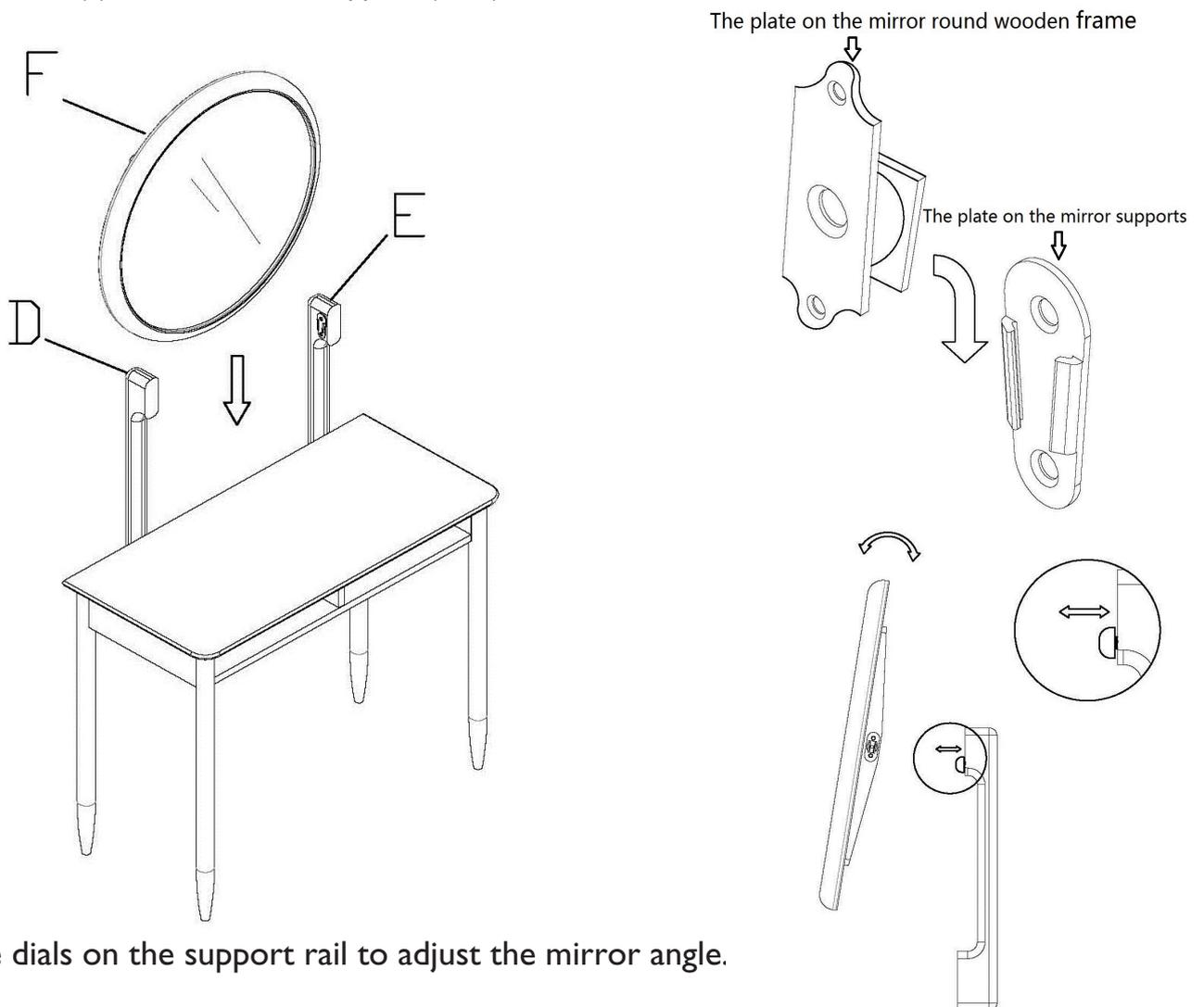
Rotate the dials on the support rail to adjust the mirror angle.
