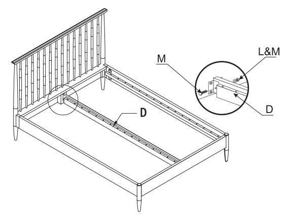
5. Push a plastic cap onto each end of a slat and with the peg facing downwards push the slat into the pre drilled holes as shown below. Repeat for all the slats.
