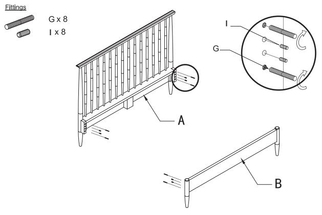
2. Making sure the holes in the side rails, C, are facing upwards, AND you have the Left and Right rails, (see page 2) on the corret sides, locate these side rails onto the protruding threads on the headboard and foot board. As you do this, slide a half moon washer onto thethread when it comes through into the circular hole in the side of the rail, then screw on one of the 8 nuts FINGER TIGHT ONLY. Repeat with the other 3 corners. then TIGHTEN FIRMLY WHEN ALL FOUR CORNERS ARE SECURED.
