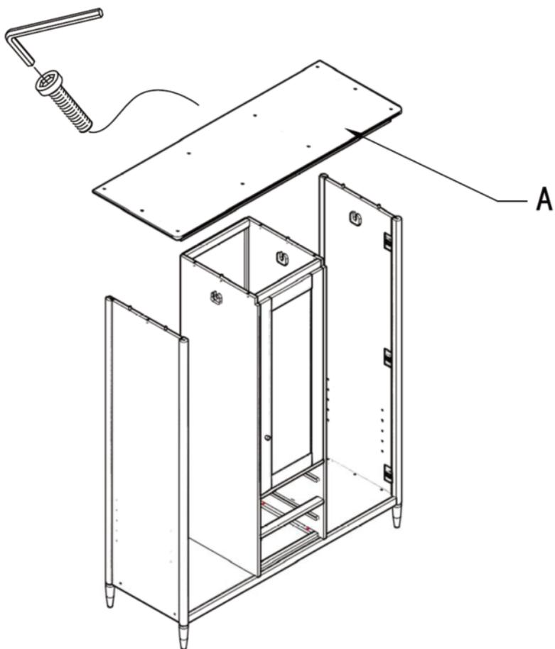
6. Using 32 of the 16mm round head screws O, attach the two back panels, H onto the back of the wardrobe.
