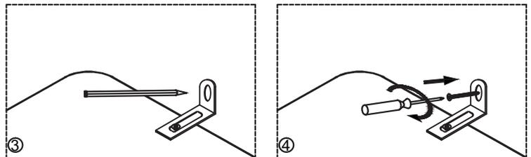
3. Mark the wall for drilling through the hole in the short face of the bracket.
