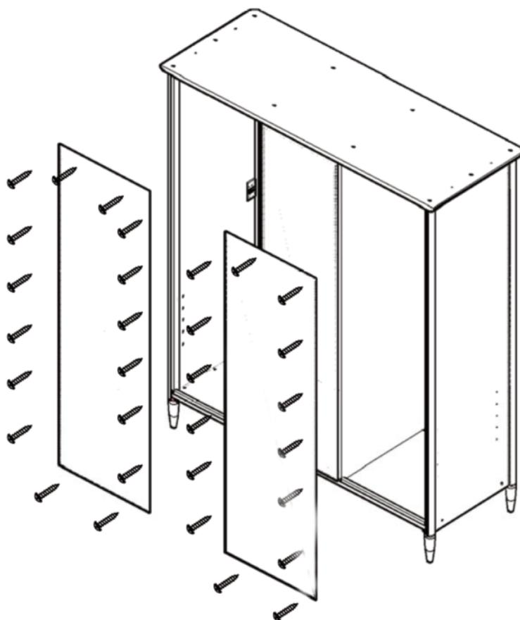
7. Using the 4x 25mm screws, N, attach the top panel to the sides through the pre drilled holes inside the wardrobe. Attach the bottom of the middle section to the bottom of the wardrobe as shown below. Then attach the L/R doors onto their hinges. Attach the door panels onto the side panels as shown below.
