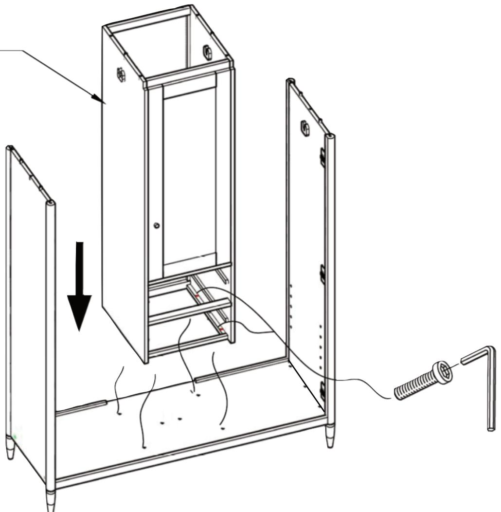
5. Using 10 allen bolts L, fix the top panel to the wardrobe as shown.
