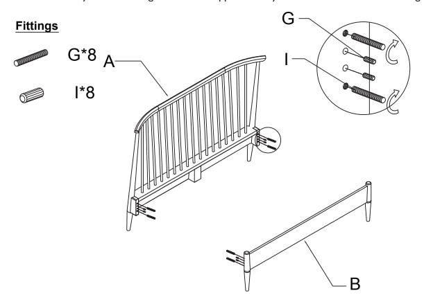
2. Making sure the holes in the side rails C, are facing upwards, AND you have the Left and Right rails, (see page 2) on the correct sides, locate these side rails onto the protruding threads on the headboard and foot board. As you do this, slide a half moon washer onto the thread when it comes through into the circular hole in the side of the rail, then screw on one of the 8 nuts FINGER TIGHT ONLY. Repeat with the other 3 corners.
