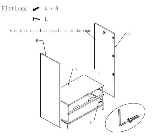
2. Attach the top panel A onto the left side panel B and right side panel C by using 8 pieces 25mm bolt K with the allen key L as shown below.
