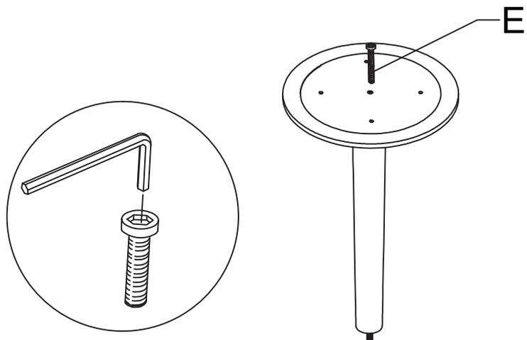
3. Attach the top panel (A) onto the column (B) using the pre-drilled bolt in the column. Twist the top panel onto the column until they are securely connected. Please see the illustration below.
