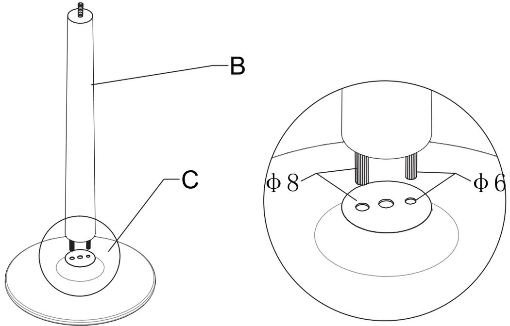
2. Use the allen key(D) to fix the the 65mm bolt (E) onto the base panel C as shown below. Tighten the bolt to make sure they are held in place well.
