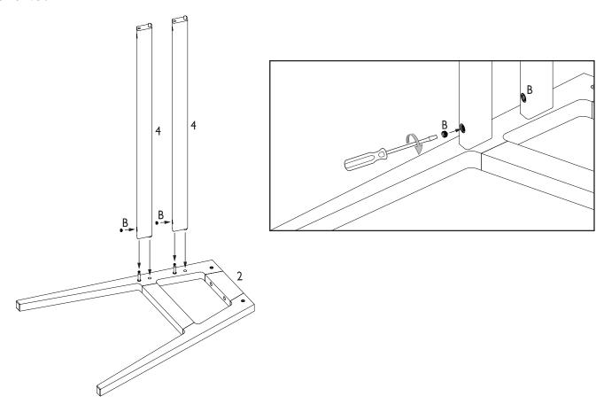
4. With the aid of an assistant, carefully attach the LH side frame (3) to the rails (4) by using 2x grub screws (B).
