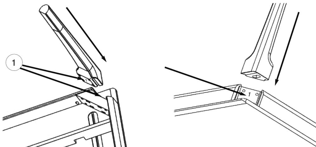
3. Put a washer onto each of four bolts and using the Allen key provided screw them into the pre bored holes as shown below. Repeat with the other three legs.
