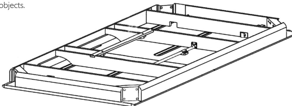
2. Each leg and corner bracket is numbered 1 to 4, slot each of the four legs into their matching corners as shown below.
