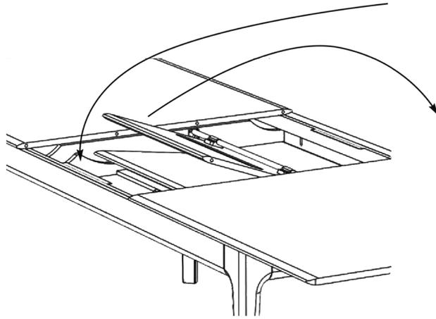
6. Lift the top flap of the butterfly extension leaves and pull it up and back over the table top as shown in the following 3 stages. As you open it the lower leaf will glide over the ramp and up into place.
