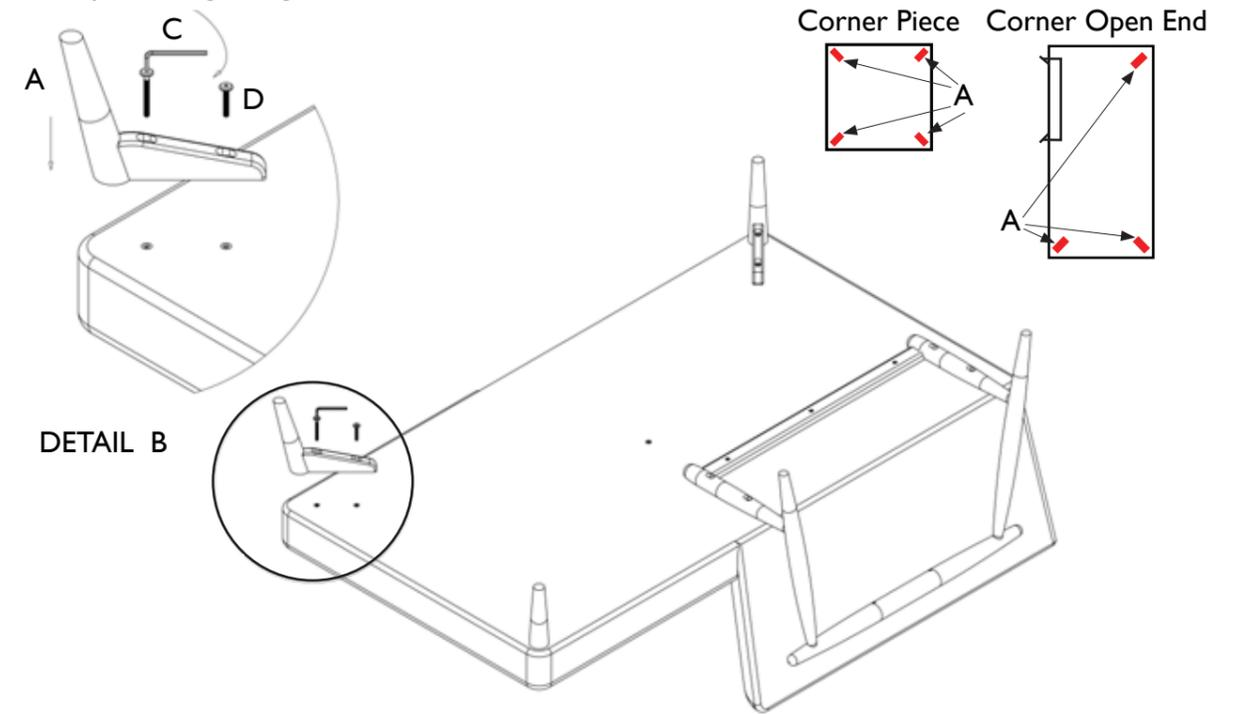
4. Following the below diagrams hand screw the adjustable legs (E) in to position (shown in **DETAIL C**).
