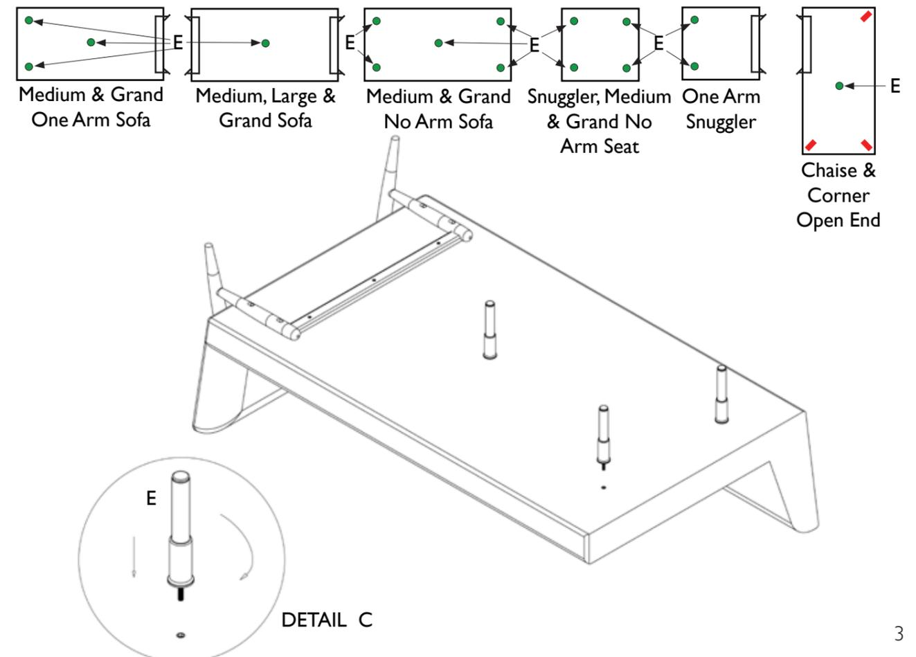
5. Carefully turn your chaise / sofa the right way up and connect the pieces as required using the linking bracket. Rotate all adjustable legs (E) ensuring they are wound out (**DETAIL D**) to be in contact with the floor.
