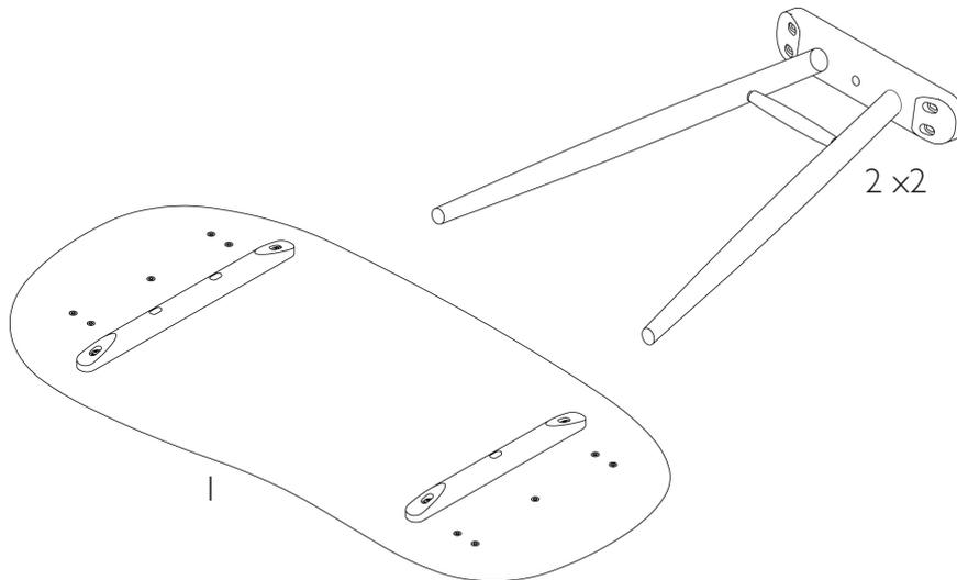
2. Take one leg assembly and align the 5 bolt holes as shown below.
