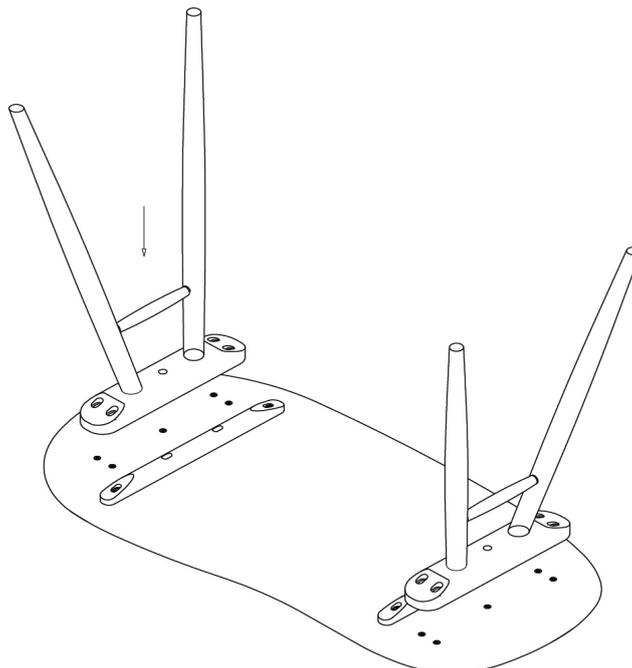
3. Take 5 x bolts (A) and using the allen key (B) tighten the bolts in a clockwise direction. Repeat with the other leg assembly.
