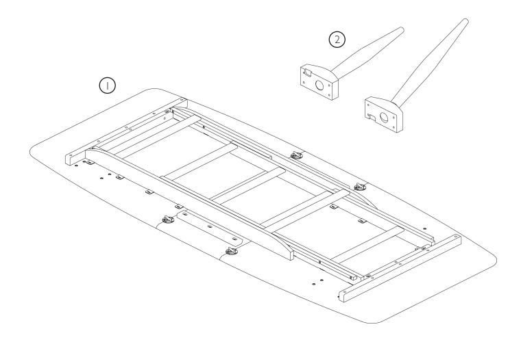
2. Take one leg assembly and align 4 bolts (A) and holes as shown below ensuring that the bracket cut out is also aligned.
