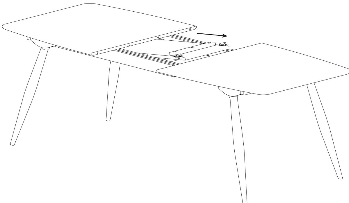
2. Place the centre leaf in position ensuring it lines up with the protruding pegs (d). Lift the table off the floor at the opposite end and slide the tops together (e).
