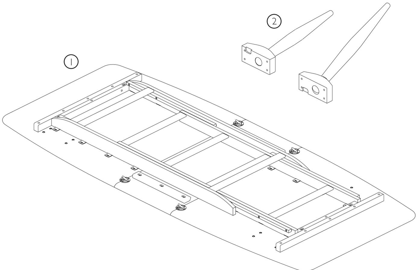
2. Take one leg assembly and align 4 bolts (A) and holes as shown below ensuring that the bracket cut out is also aligned.
