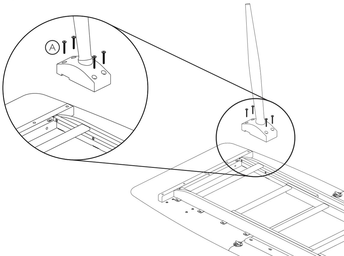
3. Using the allen key (B) fix the bolts. Repeat with the other 3 legs.
