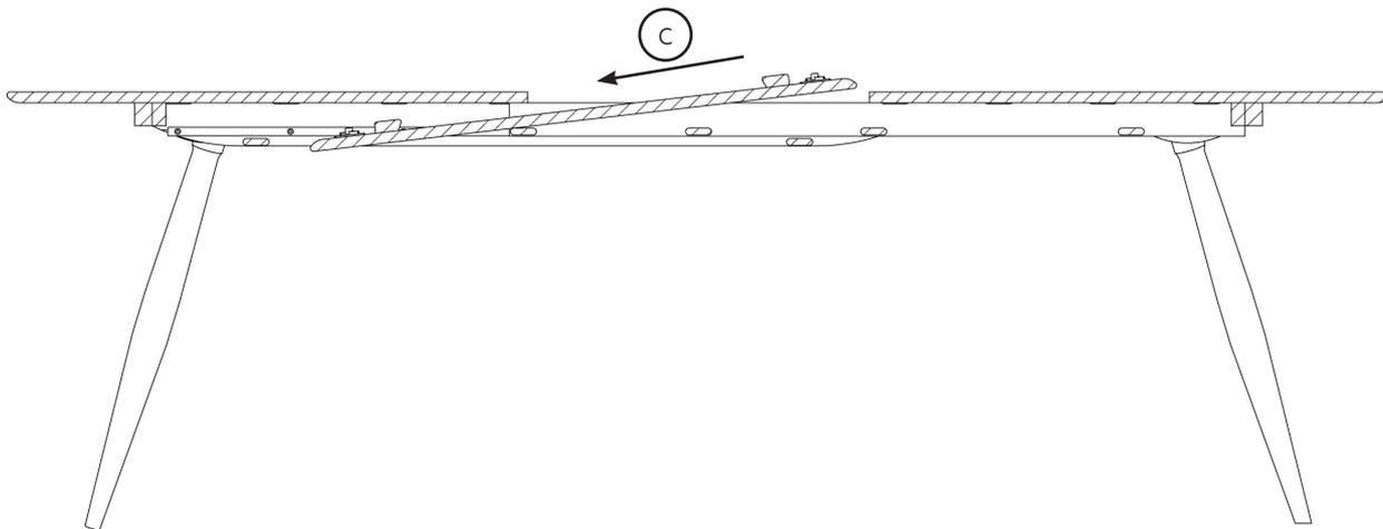
4. Rest the centre leaf on the support rails. Lift one set of legs off the ground and push the table together to close gap. Secure the table top in place by turning the catches clockwise.
