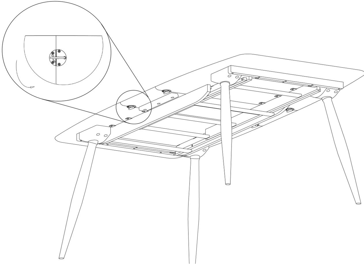
2. Lift one set of the legs off the ground and pull the table top apart (a). Lift out the centre leaf and slide on the interior support rail as shown (b).
