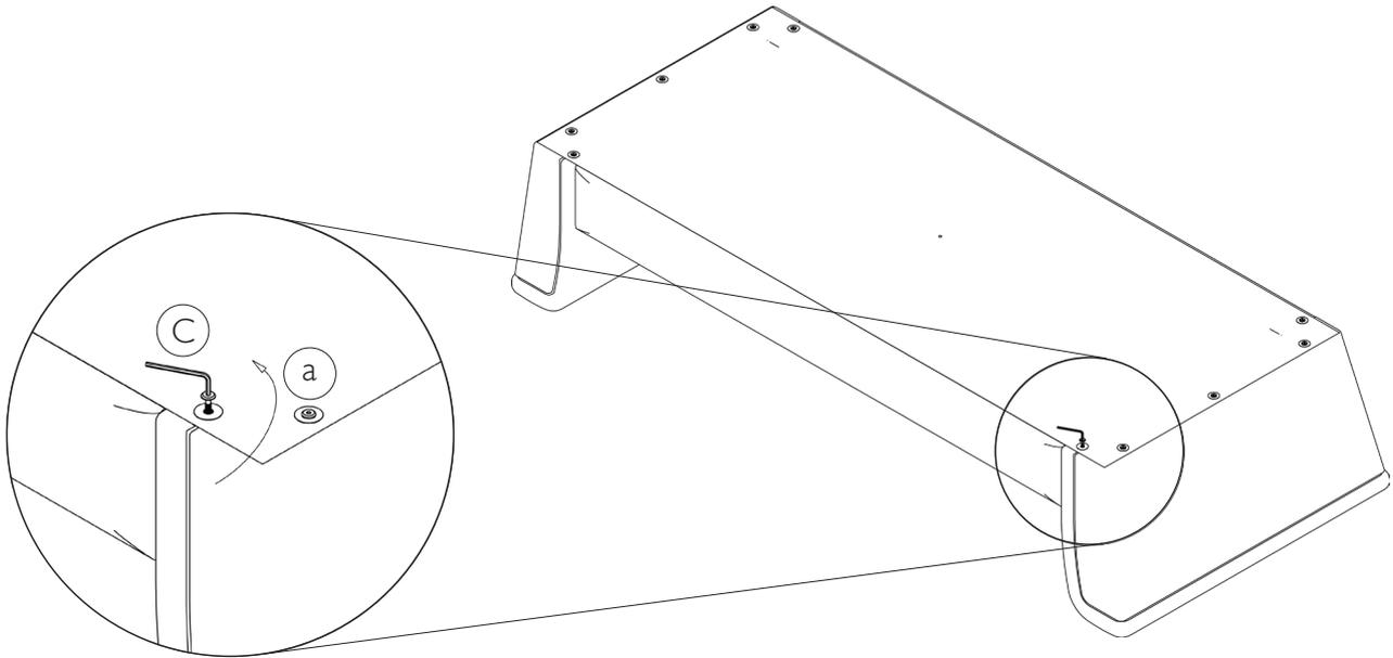
4. Take one leg assembly (A) and line up the bolts holes on the upholstery. Take 5 of the bolts (a) previously removed and insert into each hole.
