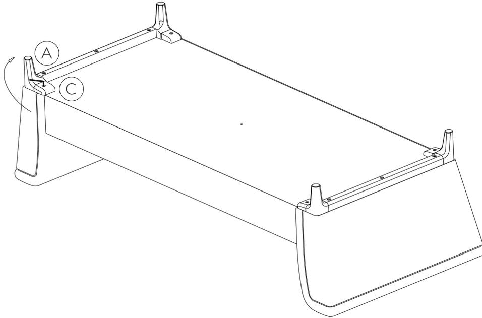
7. *Medium and Large Motion Lounger and Large Sofas only:* Take the centre leg (B) and line up with the bolt hole in the centre of the sofa. Hand tighten the centre leg by turning in a clockwise direction.
