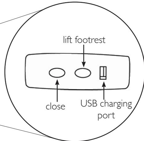
3. The footrest will rise. Release button when comfortable or continue pressing until fully extended.
