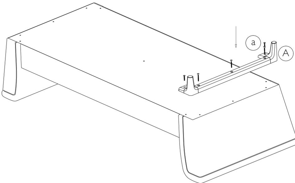
5. Tighten each bolt in a clockwise direction using the allen key provided (C).
