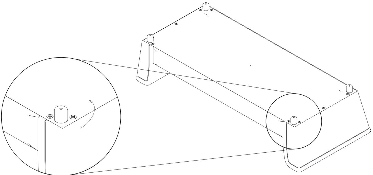
3. Using the allen key (C) undo and keep the 10 bolts (a) on the underside of the upholstery.
