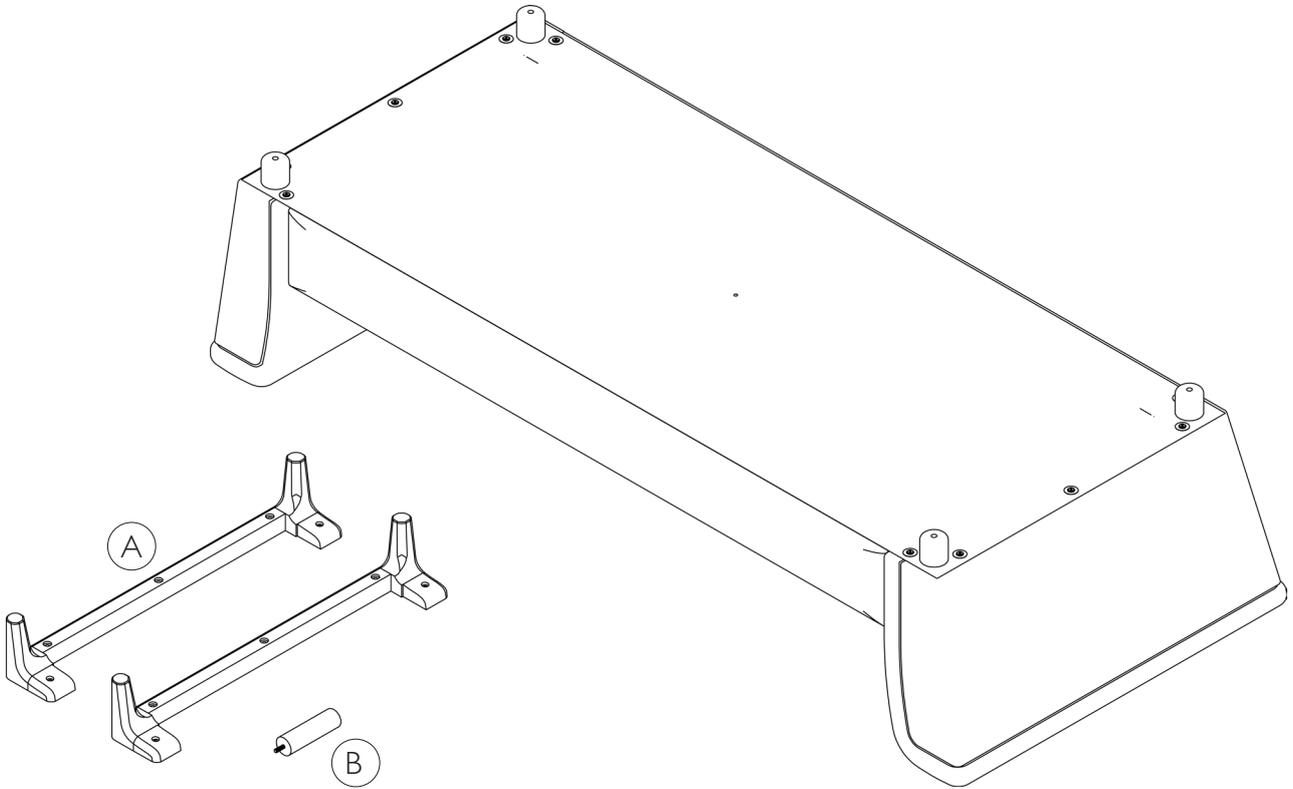
2. Unscrew the transit feet by turning anti-clockwise. Once removed these can be disposed of.
