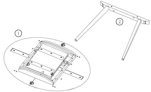
2. Undo the catches on the underside of the table top by turning anticlockwise (a).
