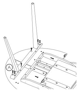
5. Using the allen key (B) fix 8 bolts by turning clockwise. Repeat with the other set of legs.
