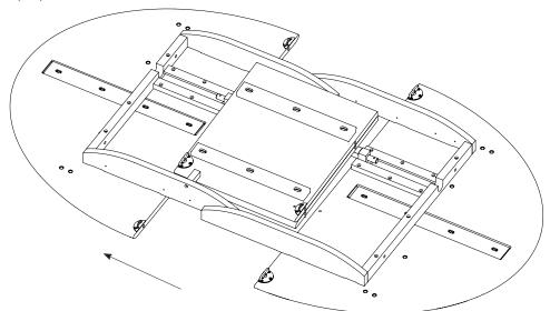
4. Take one leg assembly and align 8 bolts (A) with the holes as shown below.
