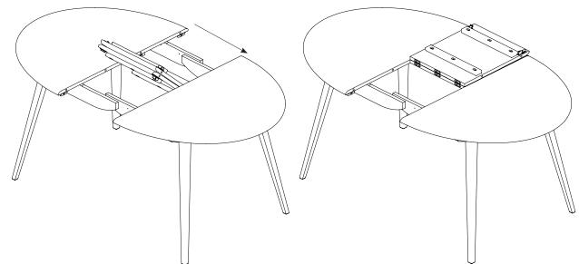
2. Lift the top flap as shown and rest on the opposite side. Fasten all four catches on the underside of the table to secure the leaves (b).
