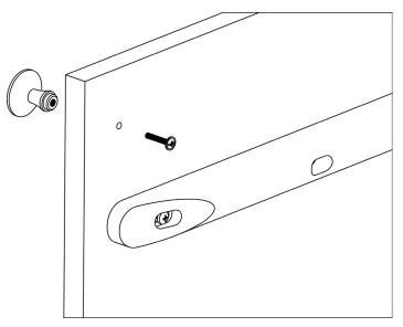
3. Using a screwdriver (not included) tighten the handle in place. Repeat with remaining handles.
